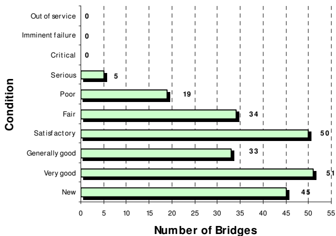
Bridge Condition Ratings
